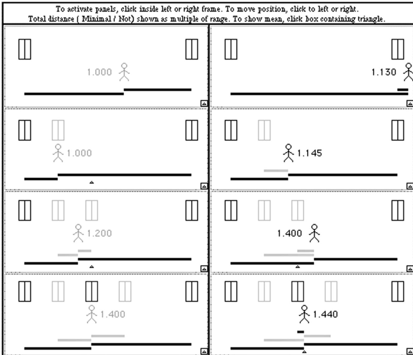
Figure 1. Total distances walked to  $n$  ( $n=2, 3, 4,$  or  $5$ ) elevators, from median (leftmost panels) and nonmedian (rightmost panels) locations. For even  $n$ , the total distance is the same from all locations between the innermost two elevators; the total distance is greater from any position outside of them; for odd  $n$ , there is only one median position which minimizes the total distance.
