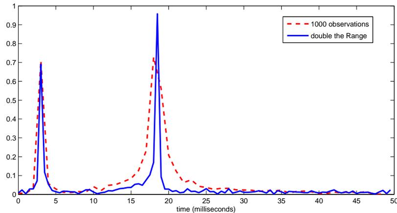
Figure 3. Fourier transform results using different observation range.
