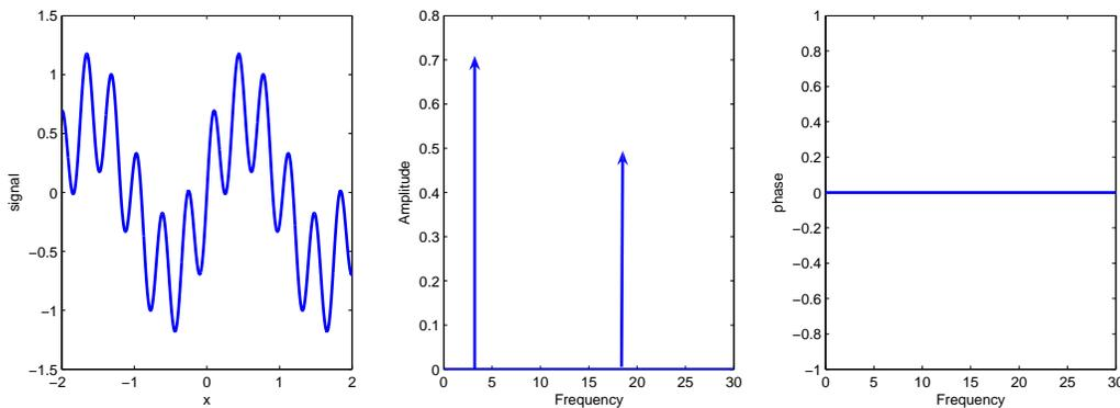
Figure 1. The amplitude (left) and phase function of the Fourier transform of  $g = 0.7 \sin(3x) + 0.5 \sin(18x)$ .
