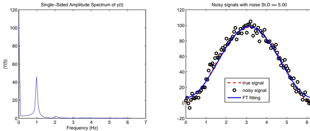
Figure 6. The FT estimation of non-trigonometric curve
