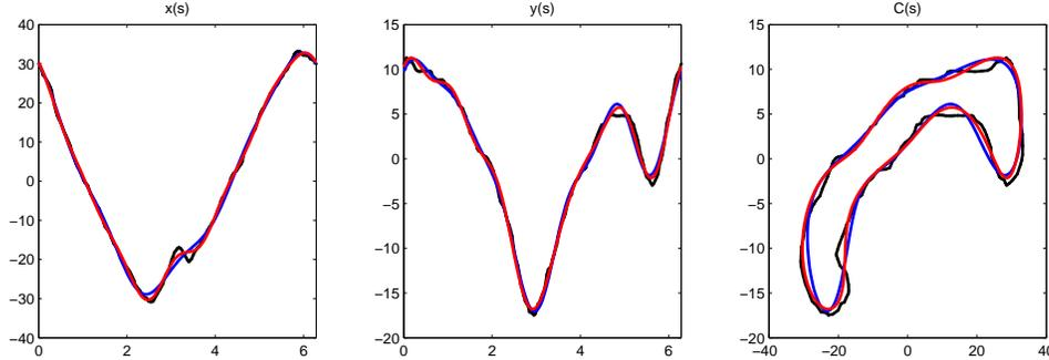
Figure 10. The reconstructed boundary of CC. The black curves are the observation, the blue curves are FT results and the LSEs of degree 6 Fourier expansion are red curves.
