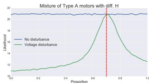
Fig. 5. In the case of motors where the only different is in the dynamic components, only a disturbance will expose the dynamic characteristic and give us information to characterize the load. Notice how the likelihood only "peaks" at the right proportion (in red) after a disturbance.
