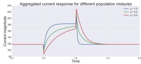
Fig. 3. Current transient for different mixtures of small and large inertia motors. Populations with higher proportion of small motors (blue) will show a faster transient.
