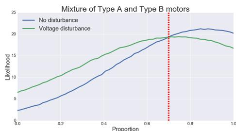
Fig. 6. Prior information allows us to have some estimate of the proportion. But it is not good due to model and measurement errors. The addition of measurements from a transient event makes our estimate better.
