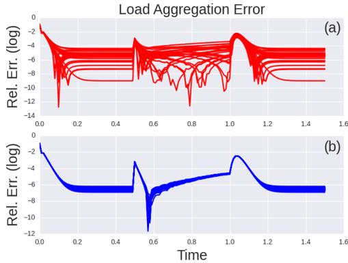
Fig. 2. The relative error for current drawn by populations of size 100 (a) and 50,000 (b) and the current drawn by the load aggregation scheme. As the population size increases, the load aggregate’s current is a better estimate of the population’s current draw because of the law of large numbers and the concentration of measure phenomenon.
