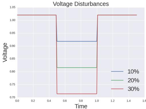
Fig. 1. The voltage profiles used in the load aggregation and estimation framework testing.
