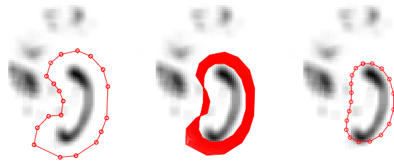
Figure 1: Left: Initial contour C_0 picked manually using ginput mouse command in MATLAB. Middle: the trace of deformation. Right: After 50 iterations with no external energy term ( \lambda = 0 ).
