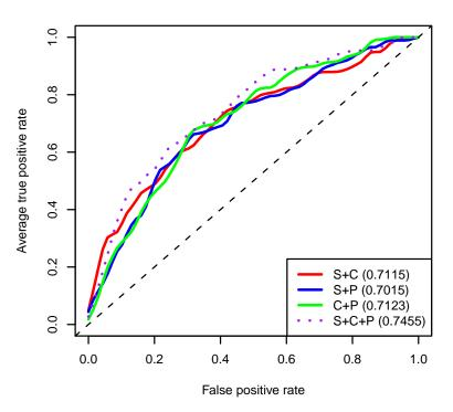
Each person in a test set is classified by thresholding their value of p(x). As the threshold goes from 0 to 1, plot "True positive rate" against "False positive rate". Dashed line-random classification.
